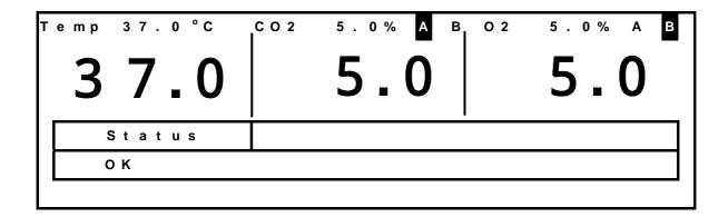
**2.** The  $N_2$  (or  $O_2$ ) gas supply line will be switched from cylinder B to A
